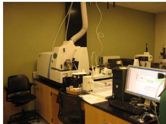
ICPMS mass spectrometer for trace analysis and student training in mass spectrometry.
